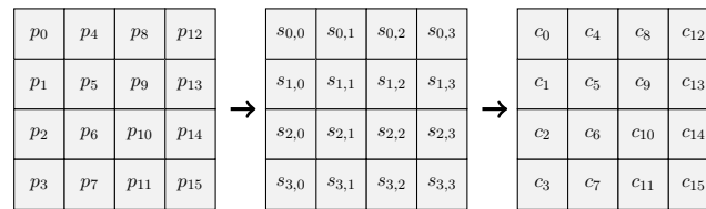
Figure 2.2: Mapping of input bytes to the State matrix and the output ciphertext
