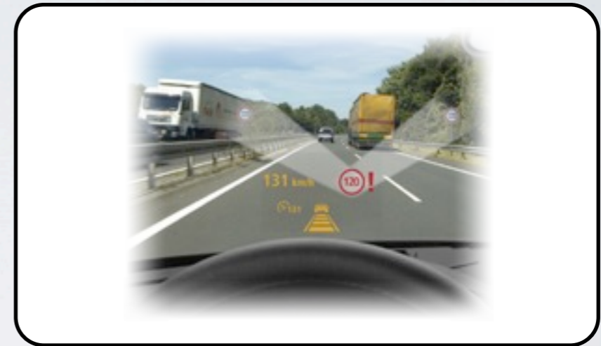
electronic traffic signs
